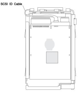
Note: On some disk drives, the SCSI ID connector on the disk drive might be different than the one shown. See the documentation that came with the disk drive for specific information about the SCSI ID connector on the disk drive.
