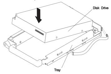
Attention: Ensure you are using the correct size screws to attach the disk drive to the tray. If the screws are longer than 5 mm (3/16 inch) you might damage the disk drive.
