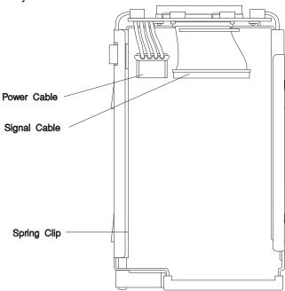
6. Install the disk drive into the tray as shown. Align the screw holes in the disk drive with the holes in the tray rails.
