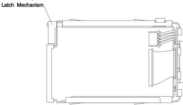
Use the following steps to assemble the Hot-Swap SCSI Disk Drive into the carrier.
